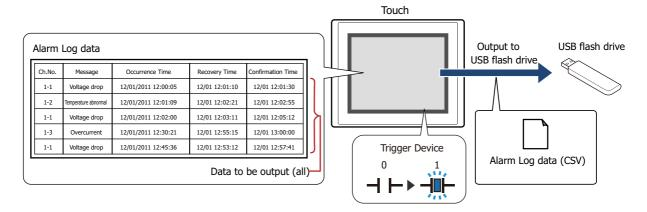
All the data is saved on the external memory when the trigger devices changes from 0 to 1. If a file with the same name already exists on the external memory, that file is overwritten. The maximum amount of output data is the amount configured by the data storage area.
