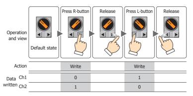
2-Notch R-return: After the knob switches from Ch1 to Ch2, it returns to Ch1 when the R-button is released.
