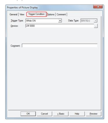
The Picture Display is enabled while the condition is satisfied, and it is disabled while the condition is not satisfied. Example: When **Trigger Type** is **While ON**, **Device** is LM0
