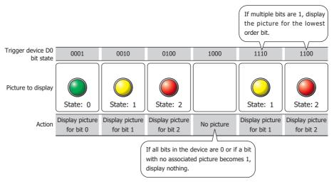
Value: Switches the drawing object displayed, according to the value of the device.
