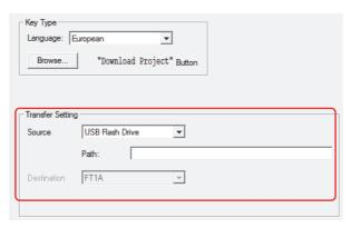
Source: This is set to the USB flash drive on which the project file to transfer (.ZNV) was saved.
