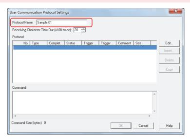
4 Set the time out (0 to 255) from when 1 frame of data has been received to when the next frame of data starts to be received in **Receiving Character Time Out (x100 msec)**.
