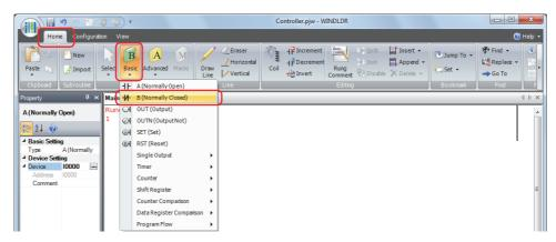
2 Move the mouse pointer to the second column of the first ladder line where you want to insert a NC contact, and then click the left mouse button.
