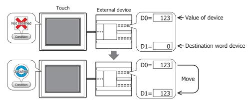
• Performs arithmetic on the value to write before writing it to a word device when the trigger condition is satisfied.
