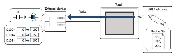
Batch read value of a device and save them to the external memory as a recipe file when a value of device changes from 0 to 1
