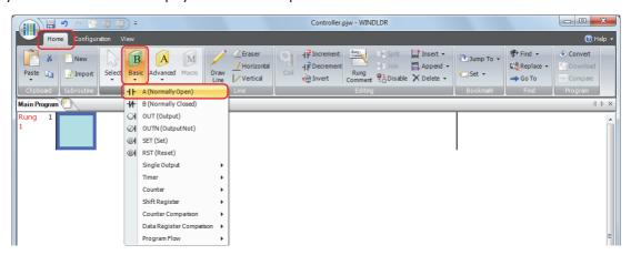
2 Move the mouse pointer to the first column of the first line where you want to insert a NO contact, and then click the left mouse button.
