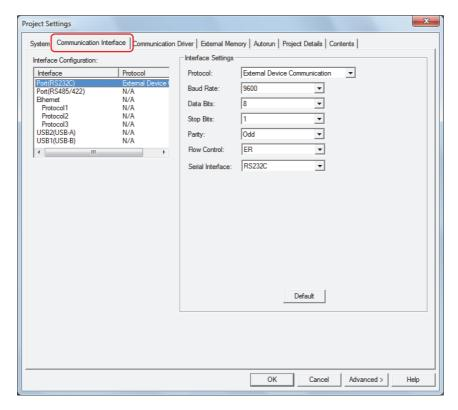
3 Select the interface for user communication under Interface Configuration, and then select the user communication in Protocol under Interface Settings.
