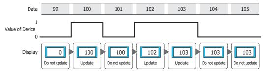
While OFF: Enables the Numerical Display when the value of device is 0.
