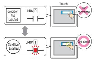
Trigger Type: Selects the condition to enable the Numerical Input from the following.
