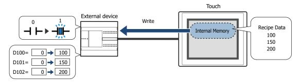
• Batch write the recipe values saved on the external memory to devices when a value of device changes from 0 to 1
