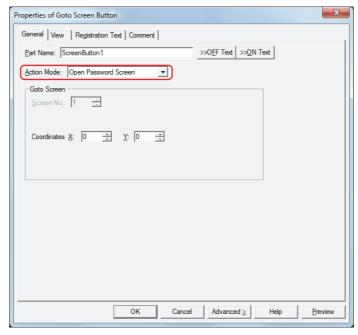
13 Specify the display location in coordinates for the password screen to open above the Base Screen with Coordinates X, Y.
