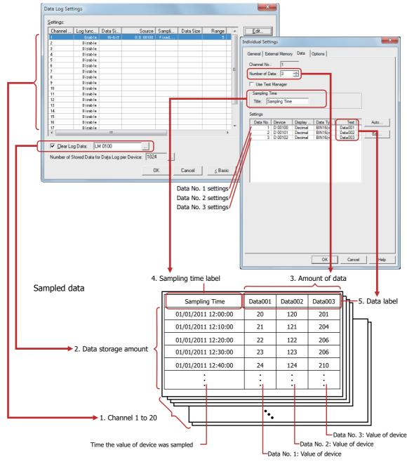
1. Channel The sampled data is in channel units. A maximum of 20 channels can be configured.
