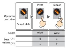
2-Notch L-return: After the knob switches from Ch2 to Ch1, it returns to Ch2 when the L-button is released.
