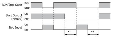
The external inputs that can be set as stop inputs are I0 to I7.
