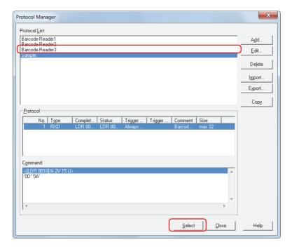
The name of the configured user communication protocol set on the **User Communication** tab in the Project Settings dialog box is displayed in **Protocol Name** under **Settings**, and the protocol settings are displayed under **Protocol**. In addition, the command settings selected under **Protocol** are displayed under **Command**.
