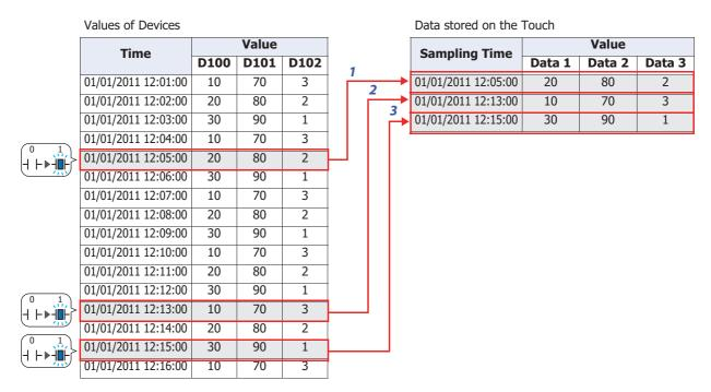
When the sampling condition device switches from 0 to 1 the fourth time, the Touch stores the values for devices D100 to D102.
