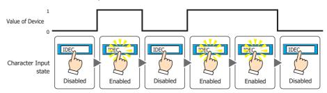
While OFF: Enables the Character Input when the value of device is 0.
