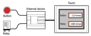
• Report the inspection time for buttons and relays by the counted operation count
