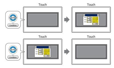
• Switches to the System Mode when the trigger condition is satisfied.
