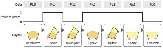
While OFF: Enables the Picture Display when the value of device is 0. Example: When **While not satisfying the condition** is **Not update Picture data**
