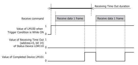
When receiving of 1 frame of data could not be completed by the time the Receiving Time Out duration elapses from when the trigger condition is satisfied, the value of the Receiving Time Out of the Status Device LDR110 (address+0, bit 14) changes to 1.
