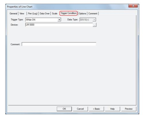
The line chart is enabled while the condition is satisfied, and it is disabled while the condition is not satisfied. When disabled, the plate and flange are displayed, but the chart is not displayed.
