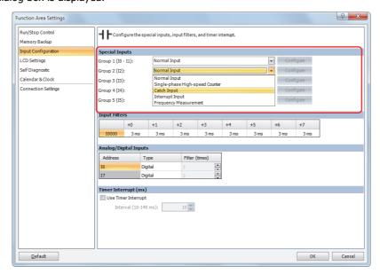
4 Select Catch Input Rising Edge or Catch Input Falling Edge in the pull-down list, and then click OK.
