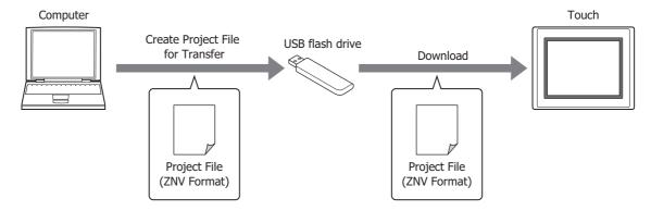
• Upload the project data used for operation on the Touch and save it to an external memory.
