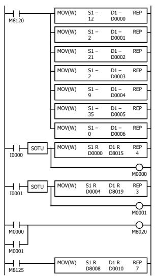
M8120 is the initialize pulse that turns on for only one scan at the start of operation.
