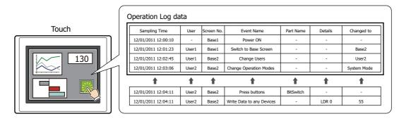
If the saved data exceeds the Operation Log data storage amount, the oldest data is deleted and the new data is saved.
