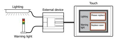
• Monitor devices connected to buttons and relays and count the operation count
