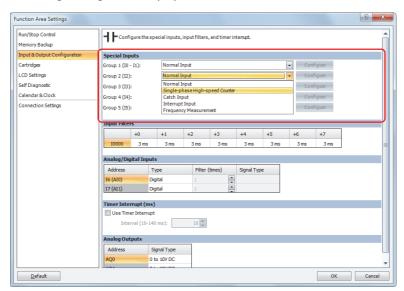
**4** Configure the operation mode and the counting mode, and then click **OK**. To use comparison actions, configure the comparison settings.
