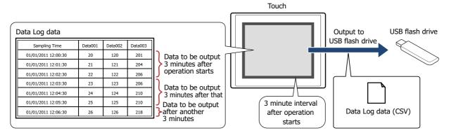
With real time output, data is saved to the external memory in three minute intervals after the Touch starts running. When there is already data with the same file name on the external memory, data is appended to that file. If there was no update to the data during the three minutes, it is not output.
