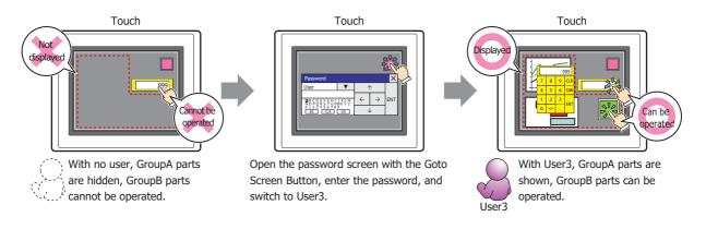
Parts that are not displayed on the screen cannot be operated regardless of the input security group.
