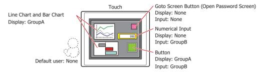
If the password screen is opened and the user switches to User2 in GroupA, the parts for GroupA are displayed. The parts for GroupB cannot be operated.
