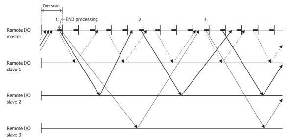
The above timing chart is an example where the communication with remote I/O slave 1 is the fastest and the communication with remote I/O slave 3 is the slowest.
