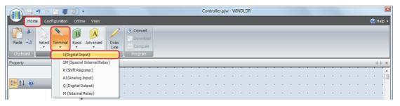
2 Move the mouse pointer to the FBD editor, and then click the mouse button. Input I0 is inserted at the position of the mouse pointer.
