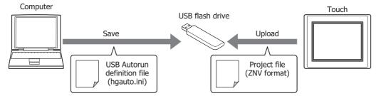
When the upload is complete, the Touch will reset and start over at the beginning of the project.
