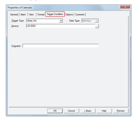
The Calendar is enabled while the condition is satisfied, and it is disabled while the condition is not satisfied. When disabled, the plate and flange are displayed, but the time is not displayed.
