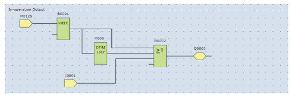
For example, in the above FBD program, the program size and the number of used devices can be calculated as described below.
