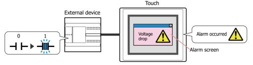
• Make a sound of the buzzer and screen flashing the screen when an alarm occurs
