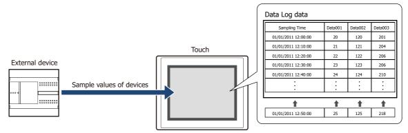
If the saved data exceeds the Data Log data storage amount per device, the old data is deleted and the new data is saved.
