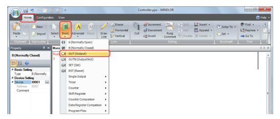
2 Move the mouse pointer to the third column of the first ladder line where you want to insert an output coil, and then click the left mouse button.
