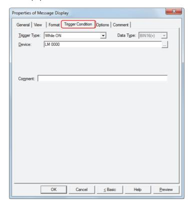
The Message Display is enabled while the condition is satisfied, and it is disabled while the condition is not satisfied. When disabled, the plate and flange are displayed, but the message is not displayed.
