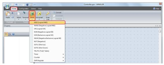
2 Move the mouse pointer to the FBD editor, and then click the mouse button. AND B0 is inserted at the position of the mouse pointer.
