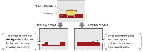
However, when the background part is the Alarm List Display, Alarm Log Display, bar chart, line chart, or pie chart, the missing sections will remain.
