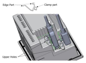
3 Fasten the USB clamp band around the USB cable and the clamp part, secure them tightly.
