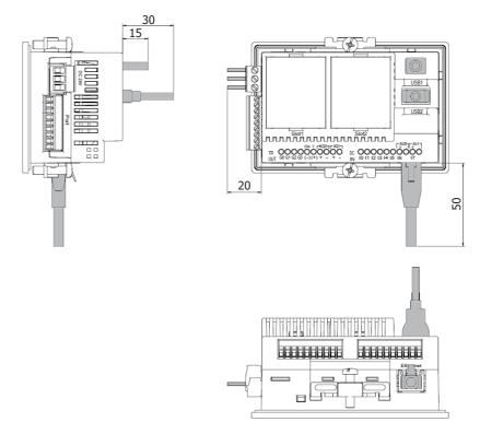
Depending on the type of connection cable used the dimensions shown above will change. The dimensions given here are intended for reference only.
