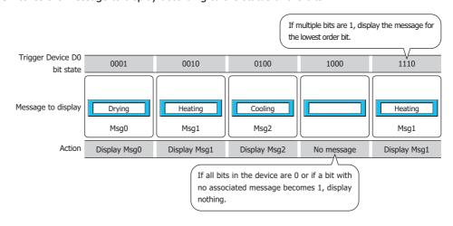
Value: Switches the message to display according to the value of device.
