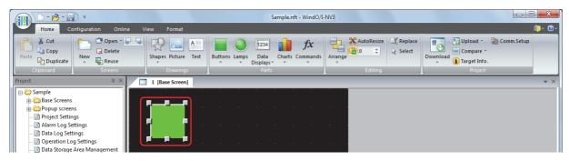
**5** Select **Switch to Base Screen** for **Action Mode**.
