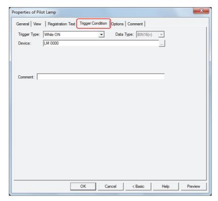
The Pilot Lamp is on while the condition is satisfied, and it is off while the condition is not satisfied. The Pilot Lamp displays the ON graphic when on and it displays the OFF graphic when off.
