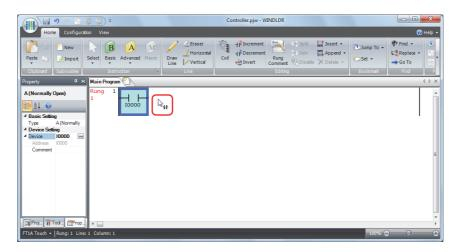
**3** Set the device in the **Property** window. Enter "I1" for **Device** and press ENTER.
