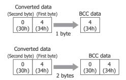
• When Calculation Type is Modbus ASCII (LCR)
