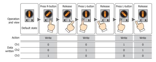
3-Notch Both-return: If the knob is switched to Ch1 or Ch3, it returns to Ch2 when the button is released.
