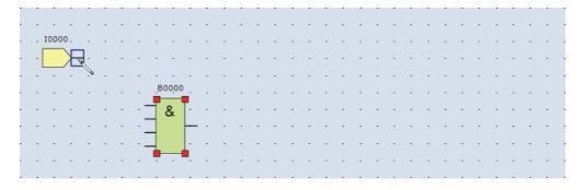
3 Click the mouse button and drag the line to the AND B0 input 1 connector.
