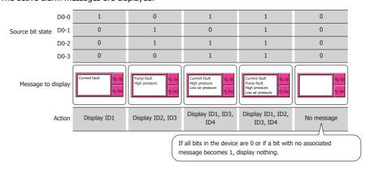
Example: When **New Message List** is selected and the bits of **Trigger Device** D0 are allocated to the following messages.
