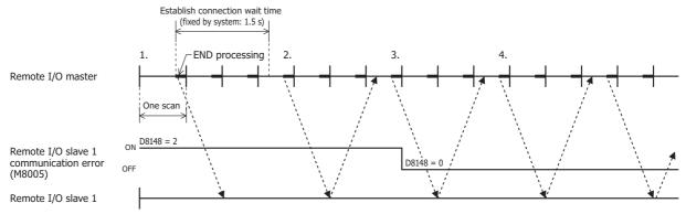
The remote I/O master issues a communication request to the remote I/O slave in the END processing.
