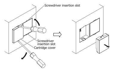
2 Pay careful attention to the direction of the cartridge and attach it directly onto the unit.
