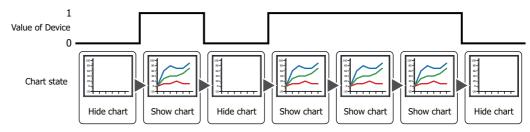
While OFF: Enables the line chart when the value of device is 0.
