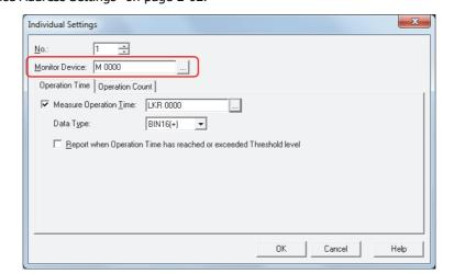
**6** Select the **Measure Operation Time** check box on the **Operation Time** tab.
