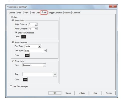
The options on the **Scale** tab vary based on the type selected with **Chart Type** on the **General** tab.
