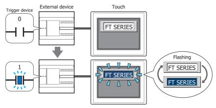
Enable: Turn this check box on to make messages flash.
