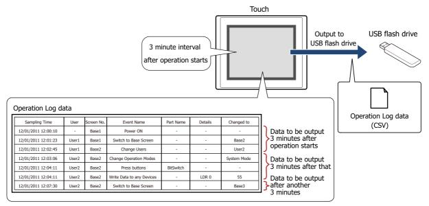
With real time output, data is saved to the external memory in three minute intervals after the Touch starts running. When there is already data with the same file name on the external memory, data is appended to that file. If there was no update to the data during the three minutes, it is not output.
