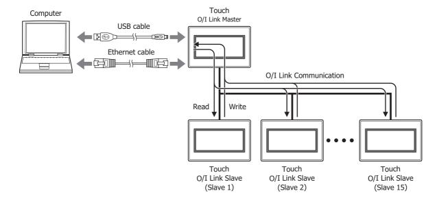
External Memory: Read or write data to the external memory inserted in the Touch connected to the computer.
