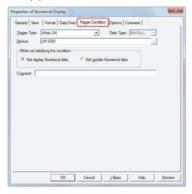
The Numerical Display is enabled while the condition is satisfied, and it is disabled while the condition is not satisfied. Select the operation when the condition is not satisfied as **Not display Numerical data** or **Not update Numerical data** under **While not satisfying the condition**.
