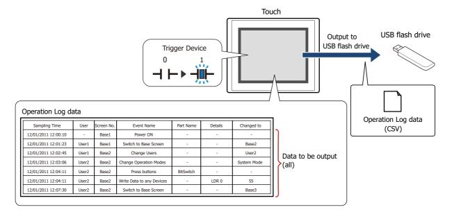
All the data is saved on the external memory when the trigger device changes from 0 to 1. If a file with the same name already exists on the external memory, that file is overwritten. The maximum amount of output data is the amount configured by the data storage area.
