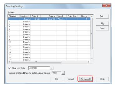
3 Under **Settings**, select the channel number for the data to display numerical values of on the Numerical Display, then click **Edit**.
