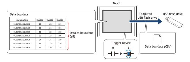
All the data is saved on the external memory when the trigger devices changes from 0 to 1. If a file with the same name already exists on the external memory, that file is overwritten. The maximum amount of output data is the amount configured by the data storage area or 1,024.
