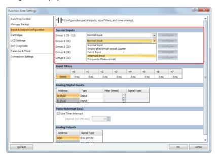
4 Select Interrupt Input Rising Edge, Interrupt Input Falling Edge or Interrupt Both Edges in the pull-down list, and then click OK.
