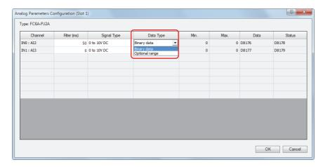
**8** If **Optional range** is selected for **Data Type**, set the minimum and maximum of analog value for each channel in the range of -32,768 to 32,767.
