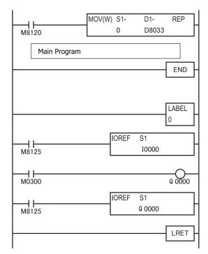
M8120 is the initialize pulse special internal relay. D8033 stores 0 to designate jump destination label 0 for interrupt input I2.
