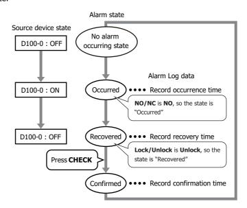
If **CHECK** is pressed before the source device changes to OFF, the alarm changes to the "Confirmed" state regardless of the state of the source device.
