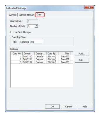
The channel number selected on the **General** tab is displayed in **Channel No.**
