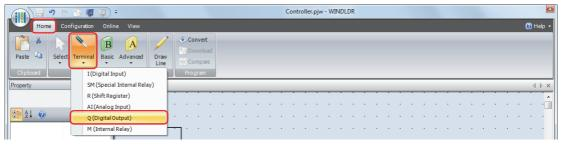
2 Move the mouse pointer to the FBD editor, and then click the mouse button. Output Q0 is inserted at the position of the mouse pointer.
