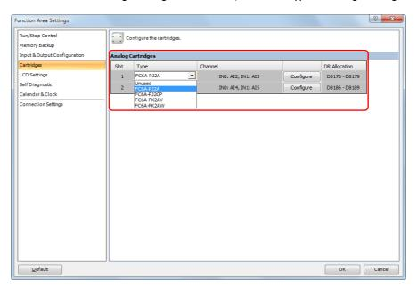
4 Click **Configure** for the **Slot** where the analog cartridge is connected.
