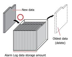
When the backup battery is depleted, the data in the Alarm Log is erased when the Touch is turned off.
