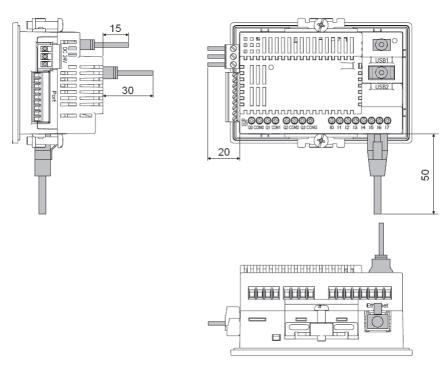
Depending on the type of connection cable used the dimensions shown above will change. The dimensions given here are intended for reference only.
