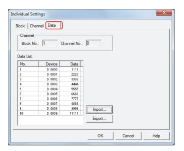
The data for the recipe in the amount specified by **Number of Data** on the **Channel** tab is configured in **Data List**. In **Device**, the devices are sequentially configured starting from the device address specified by **Top Device**.
