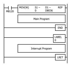
M8120 is the initialize pulse special internal relay.
