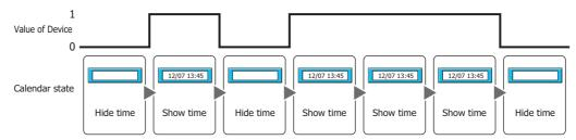
While OFF: Enables the Calendar when the value of device is 0.
