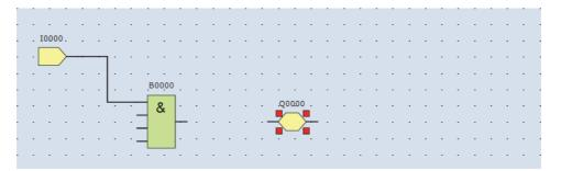
3 Connect the AND B0 output connector and the output Q0 input connector with a connection line. Connect them in the same manner as "Connect input I0 and AND B0 with a connection line" on page 12-34.
