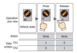
3-Notch No-return: The knob does not return when the operator's finger is released.
