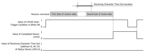
When the Receiving Character Time Out duration exceeds until the data of second byte starts to be received after the data of first byte is received, the value of the Receiving Character Time Out (address+0, bit 15) of the Status Device LDR110 changes to 1 and the Completed Device LM101 remains 0. In addition, when the value of the Trigger Condition device LM100 changes from 0 to 1, the value of LDR110 (address +0, bit 15) changes to 0.
