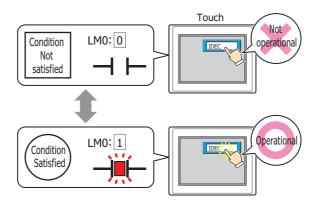
Trigger Type: Selects the condition to enable the Character Input from the following.
