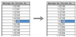
Message numbers 1-0 to 1-4 are left unchanged and screen numbers "200", "201", "202"....are automatically specified in order from message number 1-5.
