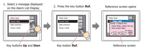
When displaying a reference screen, select either **Base Screen** or **Popup Screen** as the reference screen type. When not displaying a reference, select **Not Use**.
