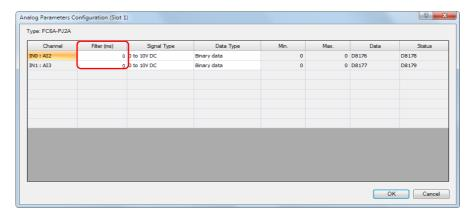
**6** Under **Signal Type**, select analog input type for each channel.
