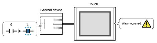
• Display an alarm screen when an alarm occurs
