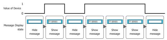
While OFF: Enables the Message Display when the value of device is 0.
