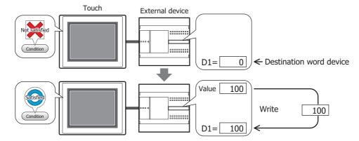
• Writes the value of device to the specified word device when the trigger condition is satisfied.
