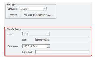
Source: Specify where to save the project uploaded from Touch. The location is the USB flash drive.
