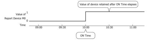
After a screen configured with the Calendar is displayed, if the time is in between ON Time and OFF
