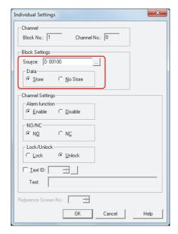
5 Select Enable under Alarm function, configure NO/NC and Lock/Unlock, and then click OK.
