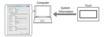
• Edit a project data in WindO/I-NV3 while checking Touch operation by displaying and changing values of devices and switching screens using the monitor function.
