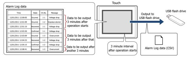
With real time output, data is saved to the external memory in three minute intervals after the Touch starts running. When there is already data with the same file name on the external memory, data is appended to that file. If there was no update to the data during the three minutes, it is not output.
