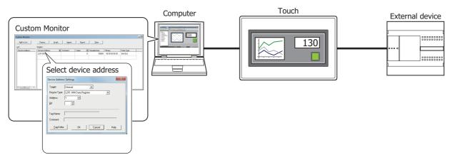
· Checking values of devices of sequential addresses
