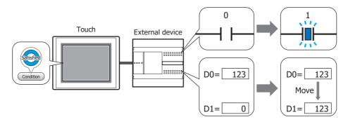
• When the trigger condition is satisfied, executes the script and switches the Base Screen.
