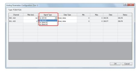
7 Under **Data Type**, select the data type for each channel.
