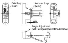
Actuator Mounting Hole Layout (horizontal/vertical swing)
