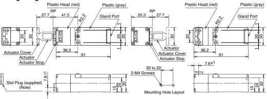
Note: Plug the unused actuator insertion slot using the slot plug supplied with the safety interlock switch.
